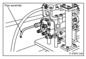
(4) Remove the CPV from cylinder B and attach the pipe assembly and the gasket.
