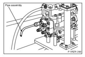
(4) Remove the CPV from cylinder B and attach the pipe assembly and the gasket.
